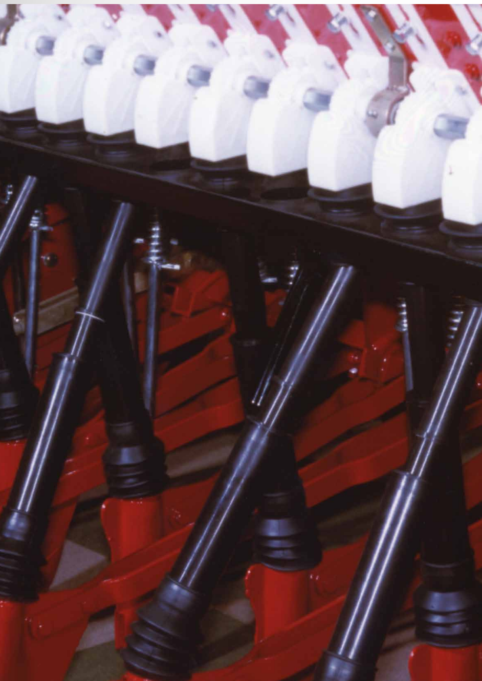
Tubo conducisemi lungo Long seed conveying tube
